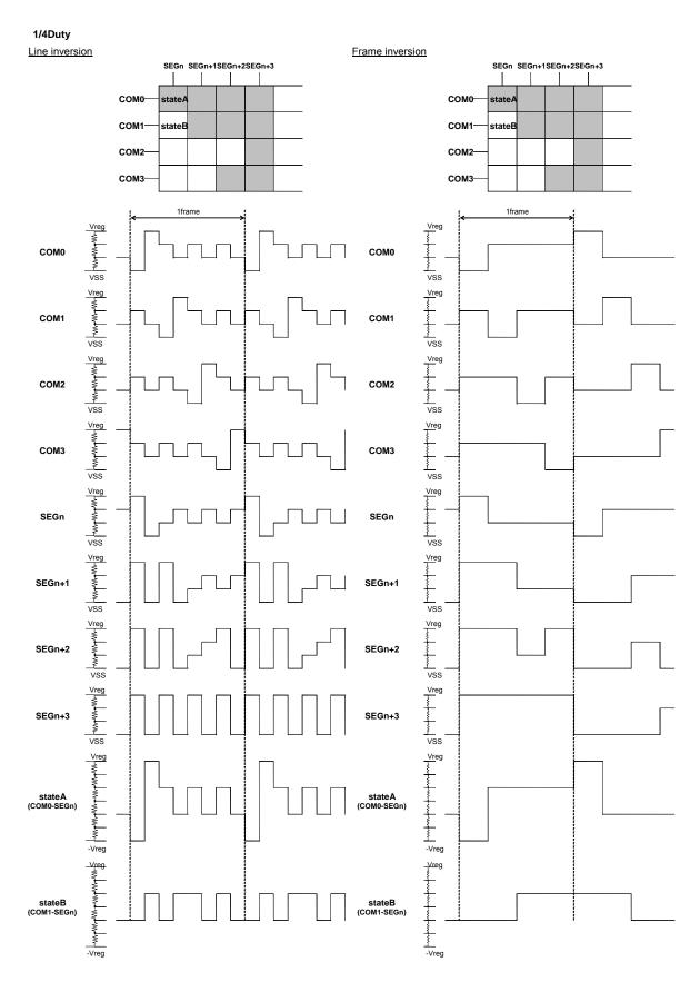
Figure 9. LCD Drive Waveform during Line inversion
