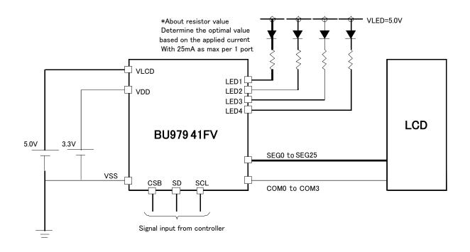
Figure 6. Recommended circuit example
