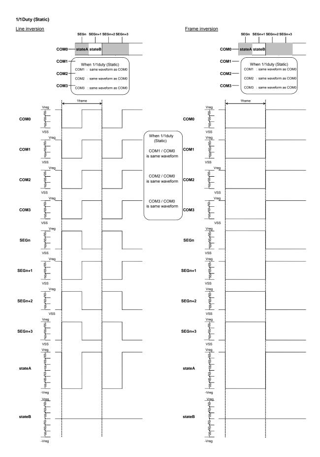
Figure 13.LCD Drive Waveform during Line inversion
