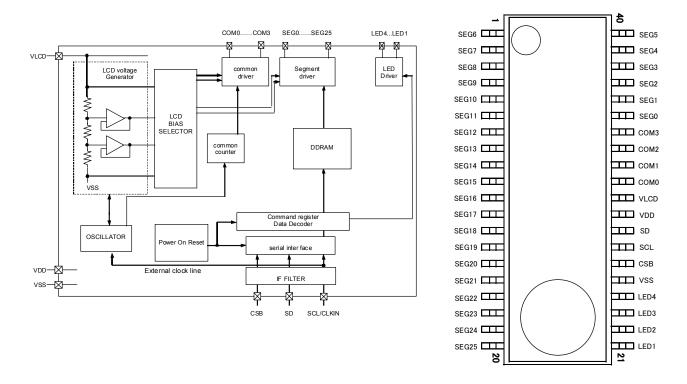
Figure 2. Block Diagram
