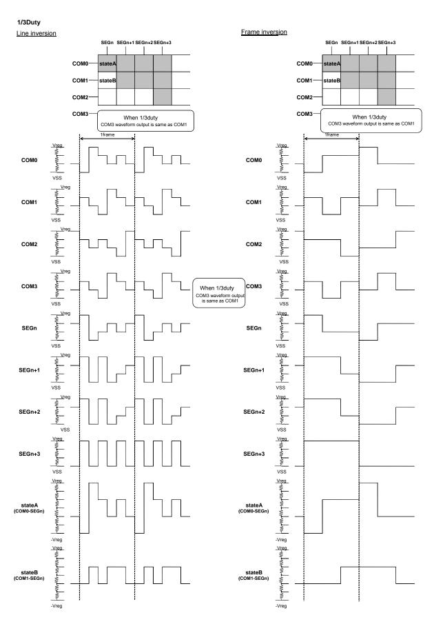
Figure 11. LCD Drive Waveform during Line inversion
