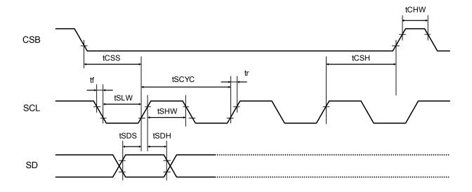
Figure 4. Serial Interface Timing
