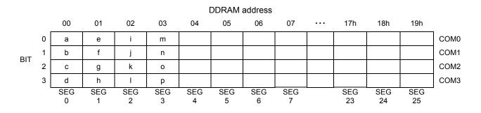
Writing to RAM is done per 4bit. When CSB is set to 'H' when less than 4bit, the writing of RAM is cancelled. (Transfer of command is done per 8bit.)
