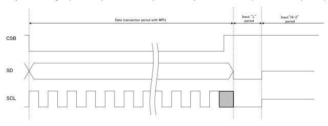
Figure 18. Recommended sequence when input ports are pulled down
