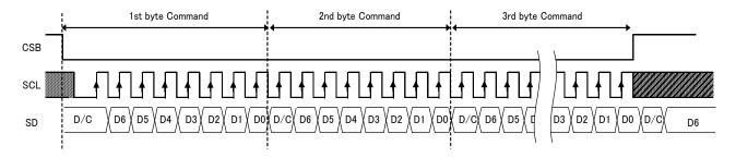
Figure 7. 3-SPI Data Transfer Format
