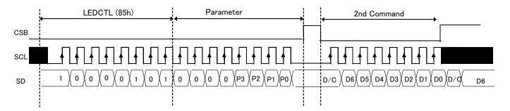
Figure 17. Recommended sequence when using LEDCTL (85h) command
